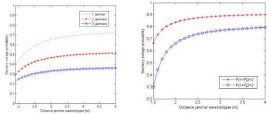
Fig 1.5 SOP under one two and three Blunt Jammers Fig 1.6 SOP under complementary energy jammers
